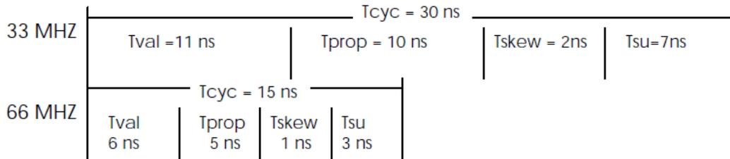
Figure 3 - PCI Timing
