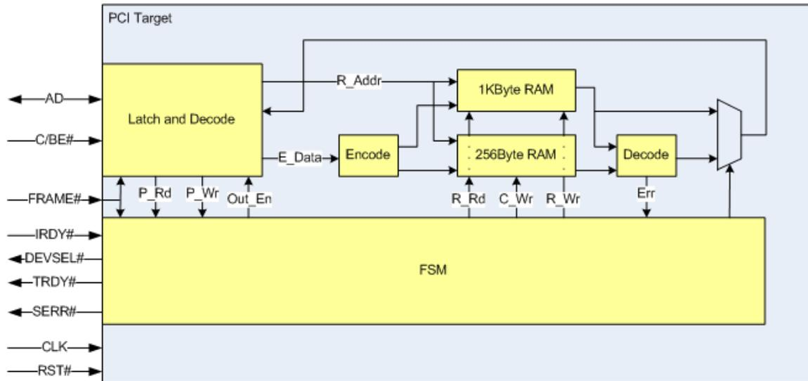
Figure 2 - Simple PCI Target with EDAC
