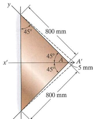
2-25. The square rubber block is subjected to a shear strain of  $\gamma_{xy} = 40(10^{-6})x + 20(10^{-6})y$ , where  $x$  and  $y$  are in mm. This deformation is in the shape shown by the dashed lines, where all the lines parallel to the  $y$  axis remain vertical after the deformation. Determine the normal strain along edge  $BC$ .
