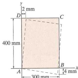
**F2-4.** The triangular plate is deformed into the shape shown by the dashed line. Determine the normal strain developed along edge  $BC$  and the average shear strain at corner  $A$  with respect to the  $x$  and  $y$  axes.
