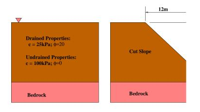
Figure 1: Clay soil deposit before and after slope is cut.
