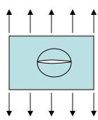
And because the stress cannot be carried through the crack, let's assume that the circular region of radius "a" around the crack has no stress in it due to the crack. The lost strain-energy due to this stress-free region is:
