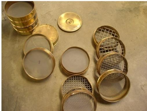
**Figure 2.1.1. Array of sieves.**
