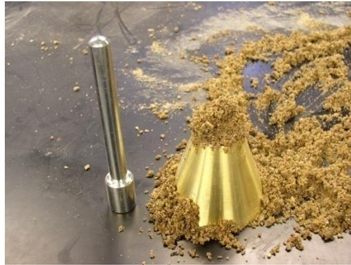
**Figure 2.1.6. Filling mold.**
