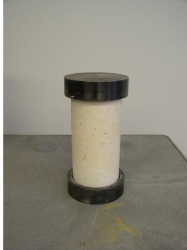
**Figure 2.3.1. Concrete specimen with caps.**
