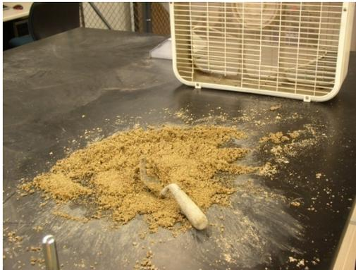
Figure 2.1.5. Drying fine aggregate to SSD.
