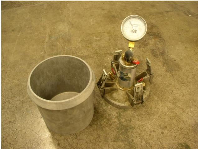
Figure 2.2.4. Air content test apparatus.
