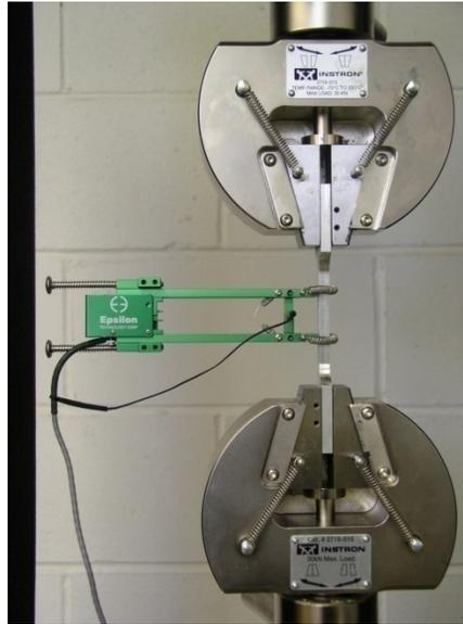
Figure 1.1.2. Specimen inserted into grips.
