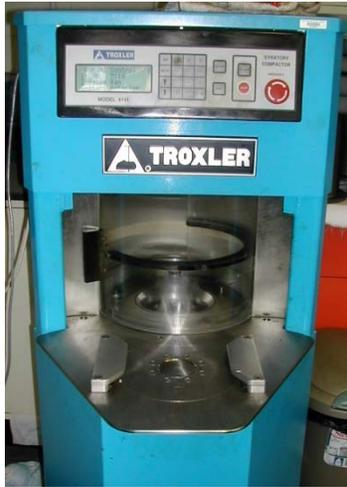
Figure 3.2.3. Troxler™ gyrotory compactor.
