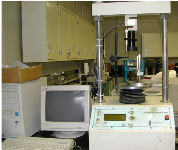
Figure 3.2.5. Split-cylinder test apparatus.
