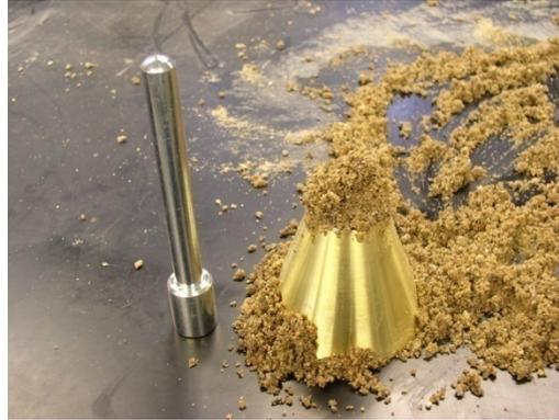
**Figure 2.1.6. Filling mold.**
