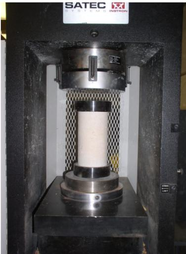
**Figure 2.3.2. Specimen in test machine.**
