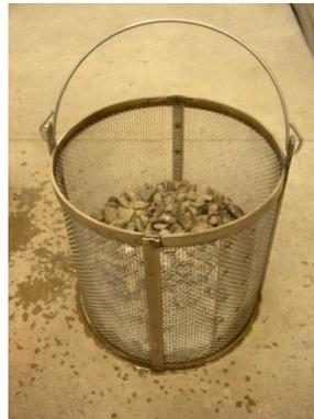
Figure 2.1.4. Aggregate in wire basket.
