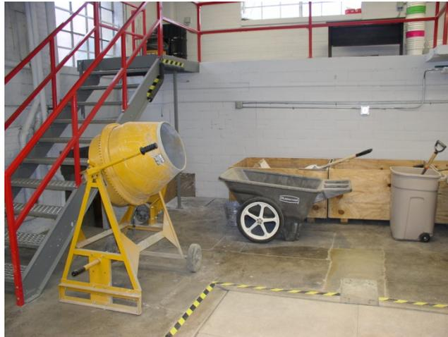
Figure 2.2.1. PCC mixing lab setup.
