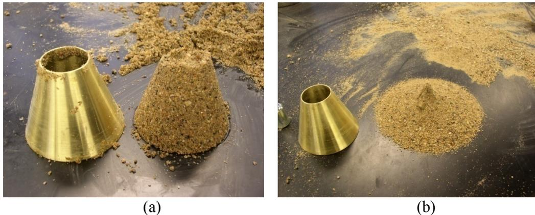
**Figure 2.1.7. Lifting mold and looking for slump.**
