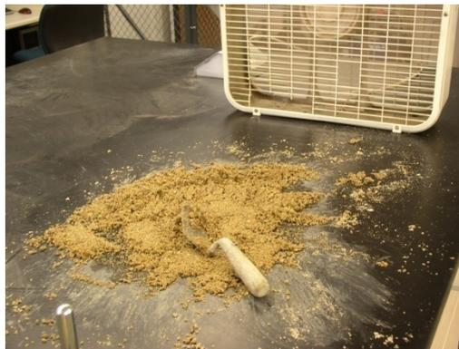
Figure 2.1.5. Drying fine aggregate to SSD.
