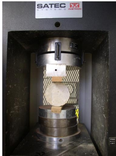
Figure 2.4.1. Specimen setup.
