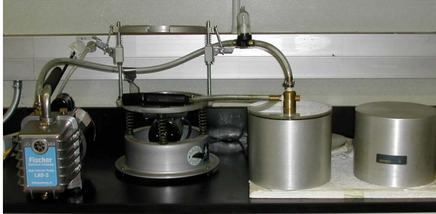
Figure 3.2.4. Rice specific gravity apparatus.
