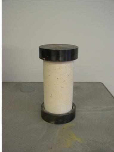
**Figure 2.3.1. Concrete specimen with caps.**
