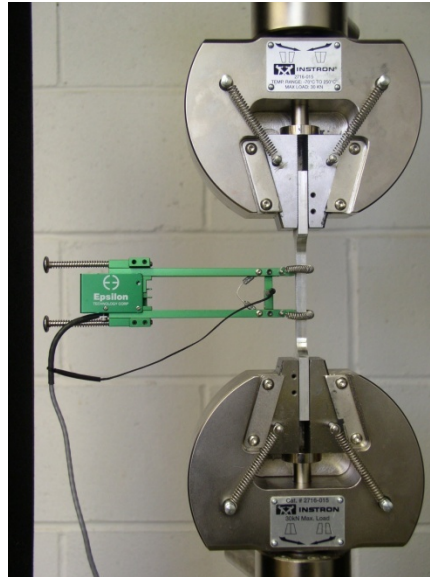
Figure 1.1.2. Specimen inserted into grips.
