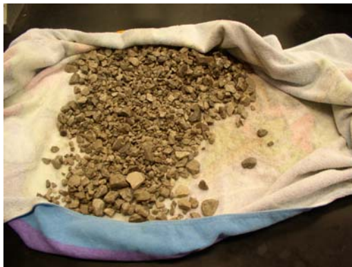
Figure 2.1.3. Towel dry aggregate.
