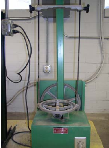
Figure 2.1.2. Small sieve shaker.
