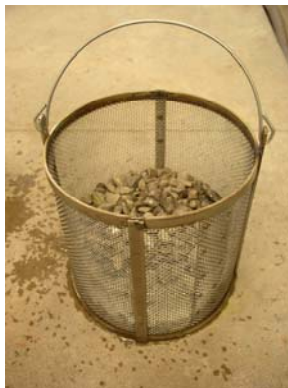
Figure 2.1.4. Aggregate in wire basket.
