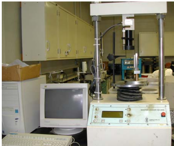
Figure 3.2.5. Split-cylinder test apparatus.
