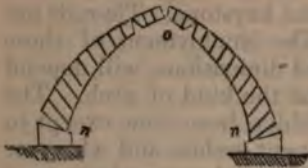
Fig. 83—Represents the manner in which pointed arches may yield. The letters refer to same points as in Fig. 82.
