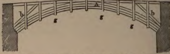
Fig. 161—Represents a wooden arch A, formed of a solid-built beam of three courses, which support the beams c, c by the posts g, g, which are formed of pieces in pairs. b, b, inclined struts to strengthen the arch by relieving it of a part of the load on the beams c, c.
