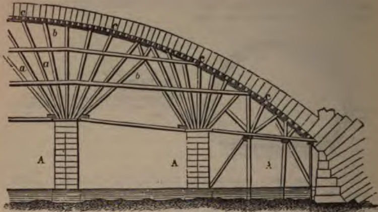
Fig. 124—Represents a part of the rib of Grosvenor Bridge over the Dee at Chester. Span 300 feet.
