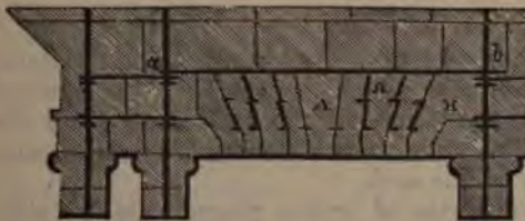
Fig. 72—Represents a cross section of a plate-bande, showing the manner in which the voussoirs A, A and B are cut and connected by metal cramps, ab , tie of wrought iron for the plate-bande fastened to the bolts cd , let into the piers of the plate-bande.
