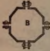
Fig. 174 A—Cross section of one of the forms of post used in a Lärville truss.
