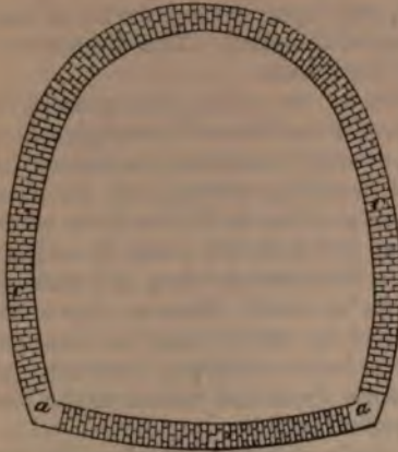
Fig. 233—Represents the general form of the cross section c of a brick arch for tunnels. a, a , askew-back stone between the sides of the arch and the bottom inverted arch.
