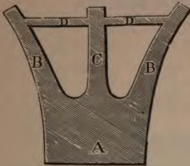
Fig. 136—Represents a horizontal section of an abutment A, with curved wing-walls B, B, connected with a central buttress C, and a cross tie-wall D.
