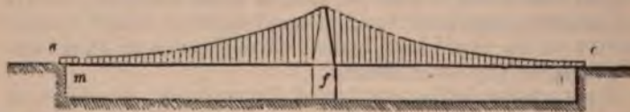
Fig. 192—Represents the manner in which the system may be arranged when a single pier is placed between the extreme points of the bearing.
