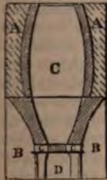
Fig. 1 represents a vertical section through the axis and centre lines of the entrances communicating with the interior of a kiln for burning lime with coal.
