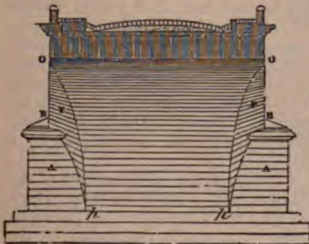
Fig. 134—Represents a cross section and elevation through the crown of Fig. 132, showing the arrangement also of the roadway, footpaths, parapet, and cornice.
