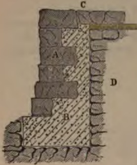
Fig. 19 is a vertical section of the sea walls used for protecting the bluffs of the islands in Boston Harbor exposed to the action of the waves.
