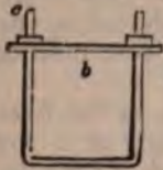
Fig. 86—Represents an iron stirrup or hoop with nuts or female screws c which confine the cross piece of the stirrup b.
