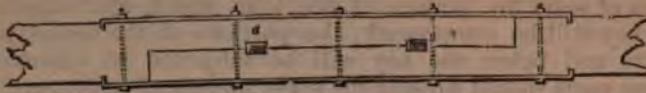
Fig. 93—Represents a scarf joint secured by iron plates c, c , keys d, d , and bolts.
