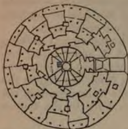
Fig. 23—Represents the manner of arranging stones of the same course by dove-tail joints and joggling, taken from a horizontal section of the masonry of the Bell-rock lighthouse.
