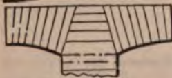
Fig. 79—Represents a mode of arranging the voussoirs and horizontal courses in flat segment arches.
