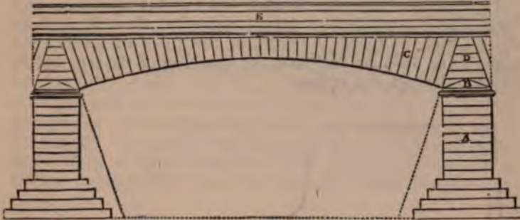
Fig. 132—Represents in elevation the combinations of the same elements as in Fig. 131 for a flat segmental arch.
