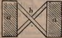
Fig. 84—Represents a cross section of horizontal beams a , a brace by diagonal battens b .
