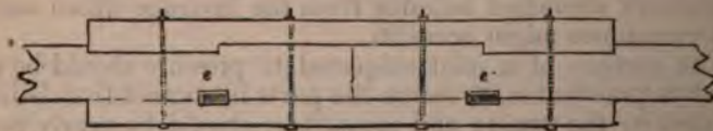
Fig. 92—Represents a fished joint in which the side pieces c and d are either let into the beams or secured by keys e , e .
