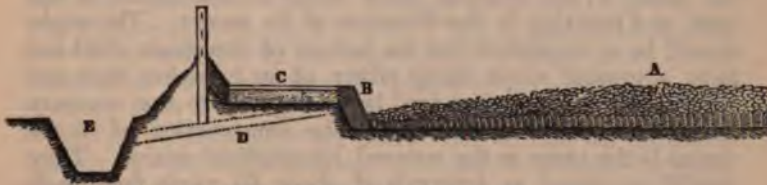
Fig. 224.—Cross-section of broken-stone road-covering.
