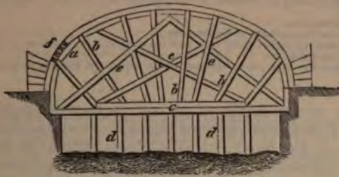
Fig. 123—Represents the rib of a centre with intermediate points of support. a , back pieces of the rib which receive the bolsters f . b, b , struts which support the back pieces. d, d , braces. c , solid beam resting on the intermediate supports d, d , which receive the ends of the struts b, b .
