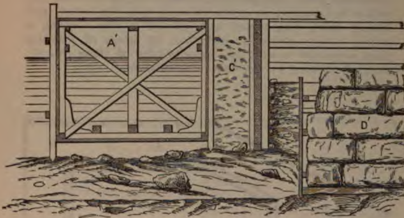
Fig. 50. Cross-section of Fig. 49. A', Cross-section of caisson.
