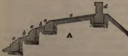
Fig. 241—Represents the method of facing the pond slope of a dam, with low walls placed in offsets.
