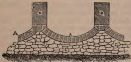
Fig. 64.—Section of vertical supports on reversed arches
