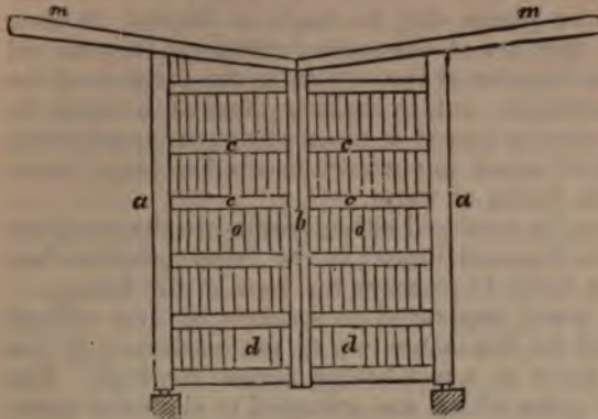
Fig. 246—Represents the elevation of a lock-gate closed. a, a , quoin-posts. b , mitre-posts. c, c , cross pieces framed into a and b , and firmly connected with them by wrought-iron plates. o , plank or sheathing of the gate. d , valve. m, m , balance-beams.
