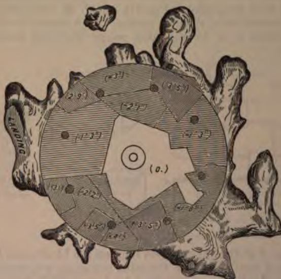
Fig. 24.—Rock surface prepared for receiving foundation.
