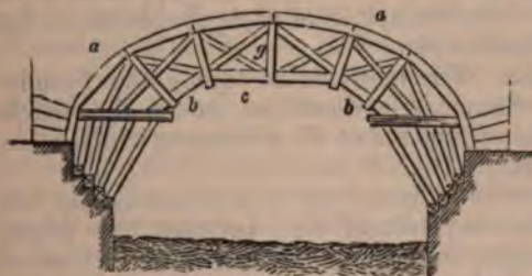
Fig. 126—Represents a frame for a rib in which the two inclined struts b, b and the straining beams c, c form intermediate supports for some of the struts that support the back pieces a, a . e, e and d are the framed extreme supports
