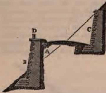
Fig. 223.—Cross section of a road in steep side-forming.
