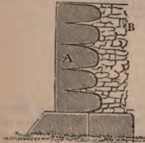
Fig. 18.—Represents a section of a wall in which the face is of cut stone, with the tails of the blocks thinned off, and the backing of rubble. A, section of face block. B, rubble backing.
