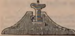
Fig. 227—Represents a cross-section a , of the fish-bellied rail of the Liverpool and Manchester Railway, and the method in which it is secured to its chair. The rail is formed with a slight projection at bottom, which fits into a corresponding notch in the side of the chair b . An iron wedge c is inserted into a notch on the opposite side of the chair, and confines the rail in its place.
