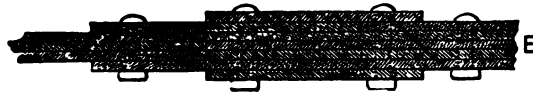
Fig. 190 C—Section of the bottom plates B of Fig. 190. There are three continuous plates and four joint plates.
