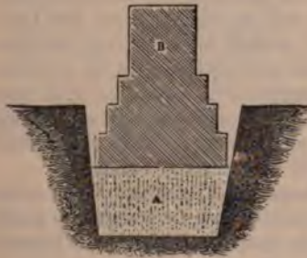
Fig. 41 represents a section of a sand foundation bed and the masonry upon it. A, sand bed in a trench. B, masonry.
