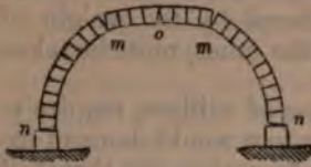
Fig. 82—Represents the manner in which flat arches yield by rupture. o, joint of rupture at the keystone. m, m, joints of rupture below the keystone. n, n, joints of rupture at springing lines.
