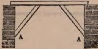
Fig. 100—Represents a horizontal beam C supported near the middle by inclined struts A, A .
