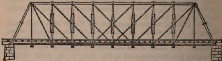
Fig. 167.—The upper chord is of cast-iron and made in sections, the length of each piece being equal to the length of a bay. The lower chord is composed of a succession of links (see Fig. 168), which receive cast-iron blocks at their ends. The cast-iron blocks form steps for securing the lower ends of the vertical posts. The posts have openings near the middle of their length, through which the main and counter-ties pass. The posts are trussed at the middle, as shown in the figure.
