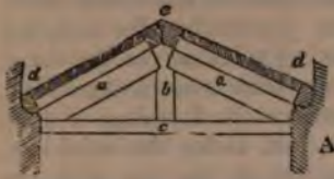
Fig. 245—Represents a plan of a wooden mitre-sill, and a horizontal section of a lock-gate (Fig. 246) closed. a, a , mitre-sill framed with the pieces b and c , and firmly fastened to the side walls A, A . d , section of quoin posts of lock-gate. e , section of mitre posts.
