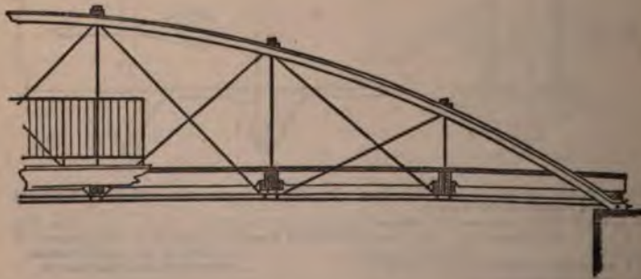
Fig. 175—An Arched Truss after the general plan of Whipple's. The lower chords or tie rods pass through the ends of the arch, and are secured by nuts on the ends of the rods.
