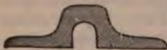
Fig. 230—Represents a cross-section of the rail of the Great Western Railway in England. This rail is laid on a continuous support, and is fastened to it by screws on each side of the rail. A piece of tarred felt was inserted between the base of the rail and its support.
