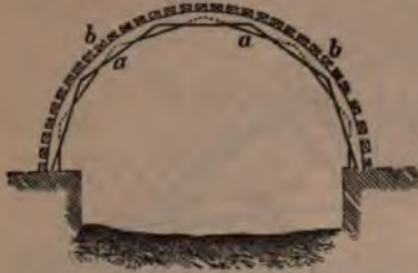
Fig. 122—Represents the rib of a centre for light arches. a, a , rib formed of planks. b, b , bolster pieces which receive the masonry.
