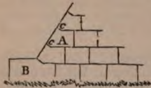
Fig. 17—Represents the arrangement of stone with abutting, or elbow joints for very inclined surfaces.
