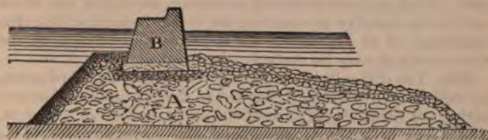
Fig. 248—Represents a section of the Cherbourg breakwater. A, mass of stone. B, battery of masonry.
