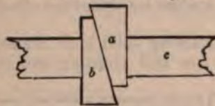
Fig. 90—Represents the keys in the form of double, or folding wedges a, b let into a shallow notch in the beam c.
