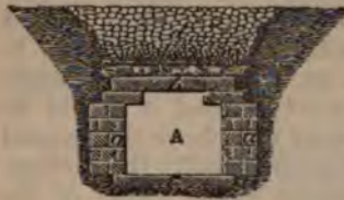
Fig. 225.—Cross-section of a covered drain. A, drain. a, a, side walls. b, top stones. c, bottom stones. d, broken stone or large gravel laid over brush.
