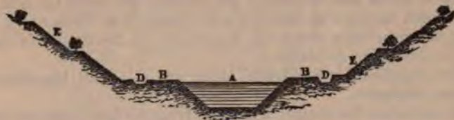
Fig. 238.—Cross section of a canal in deep cutting. E, side slopes of cutting.
