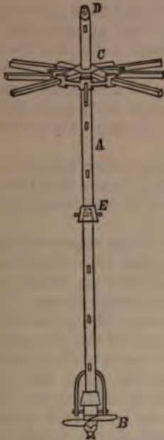
Fig. 88 represents the capstan for driving screw piles by hand.
