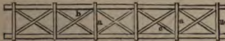
Fig. 99—Represents an open built beam; A and B are the top and bottom rails or strings; a, a, cross pieces, either single or in pairs; b, diagonal braces in pairs; c, single diagonal braces.
