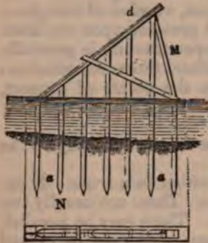
Fig. 149—Elevation M and plan N of a simple ice-breaker. a, a, foundation piles. b, b, capping of piles. c, c, uprights. d, inclined fender-beam shod with iron.
