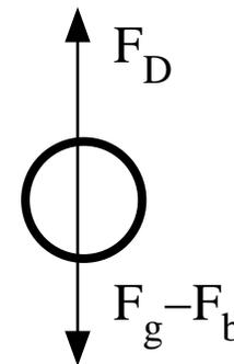
$$F_g - F_b = (1/6)(G_s - 1)\gamma_w \pi D^3 \text{ where: } G_s \text{ is the specific gravity of the soil grain and } \gamma_w \text{ is the unit weight of water (kN/m}^3\text{)}$$
