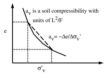
• Putting it all together, the final statement of fluid mass conservation is:  $(k_z/\gamma_w) \partial^2 u/\partial z^2 = [a_v/(1+e_0)] \partial u/\partial t$
