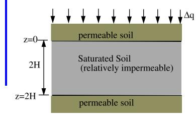
Initial conditions for excess pore-pressure in the low-permeability soil layer:  $u = u_0 = \Delta q$  for  $z \in (0,2H)$  at t=0
