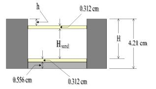
Once the mass and the height of the soil sample have been determined, the void ratio  $e_0$  can be easily computed using the following equations.
