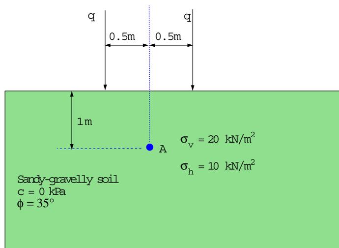
**Figure 1.** Soil deposit with initial stresses at point A, and line loads from rails.
