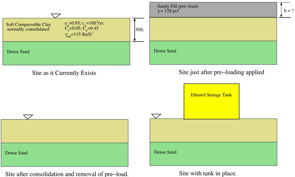
**Figure 3.** Existing site and proposed construction sequence.
