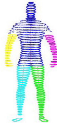
Figure 3-18: Ray casting automated segmentation result [8]. The horizontal transitions between the torso, arms, and legs make it difficult to animate the mannequin without experiencing significant overlap or gaps that are difficult to patch without more complex methods.
