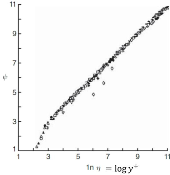
**Figure 7.20**  $\psi$  vs.  $\log y^+$  where  $\eta \equiv y^+$  in this figure. Data are taken from 16 different Reynolds numbers from  $4 \times 10^3$  to  $3.24 \times 10^6$  measured in [29]. From [31]. Reprinted with permission from ASME International.
