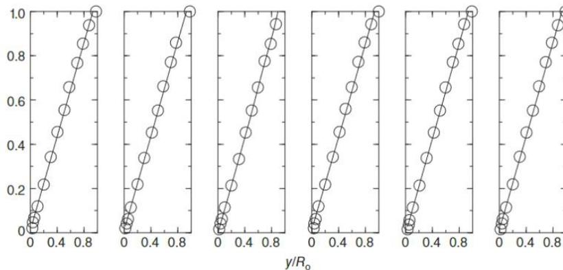
Figure 7.19 Plots of  $(\bar{U}/\bar{U}_{max})^{1/n}$  in pipe flow for empirically fitted exponents,  $n$ . From left to right  $n = 6.0, 6.6, 7.0, 8.8, 10.0$ , and the Reynolds numbers are  $4 \times 10^3, 2.3 \times 10^4, 1.1 \times 10^5, 1.1 \times 10^6, 2 \times 10^6$ , and  $3.2 \times 10^6$ . From [25], p. 563.
