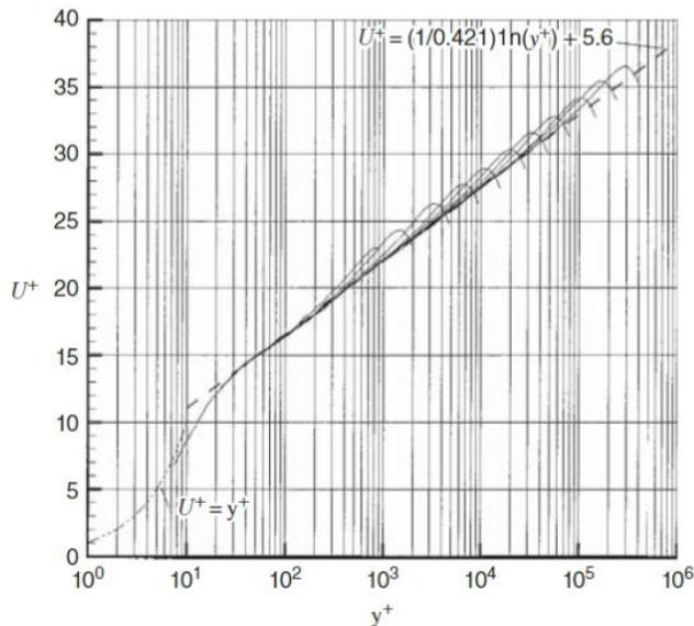
Figure 7.18 Mean velocity profiles in pipe flow [6] showing the collective approach to a log law. The curves are for Reynolds numbers between  $R_e = 31 \times 10^3$  and  $R_e = 18 \times 10^6$ . Reprinted with permission of Cambridge University Press.
