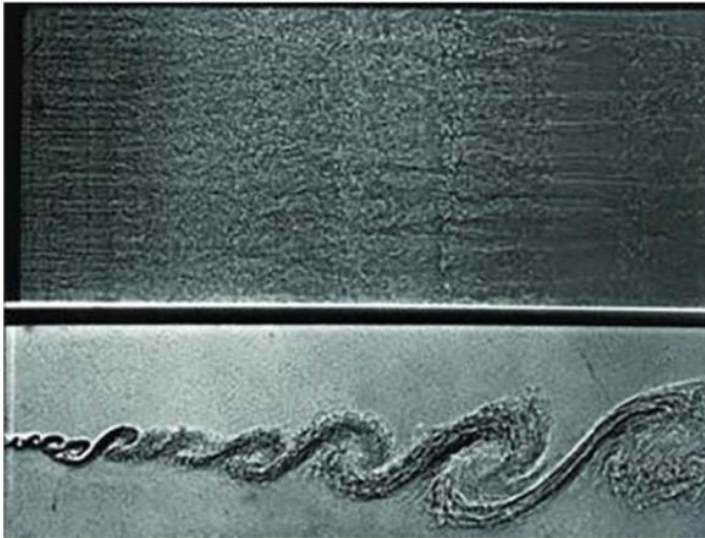
Figure 11.9 Growth of a turbulent mixing layer with x , y , and z denoting the streamwise, cross-stream, and spanwise coordinates, respectively. Top: viewed from above ( x - z ) plane; bottom: viewed from the side ( x - y ) plane. From [15].
