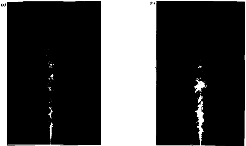
Fig. 1.2. Planar images of concentration in a turbulent jet: (a) Re = 5,000 and (b) Re = 20,000 . From Dahm and Dimotakis (1990).
