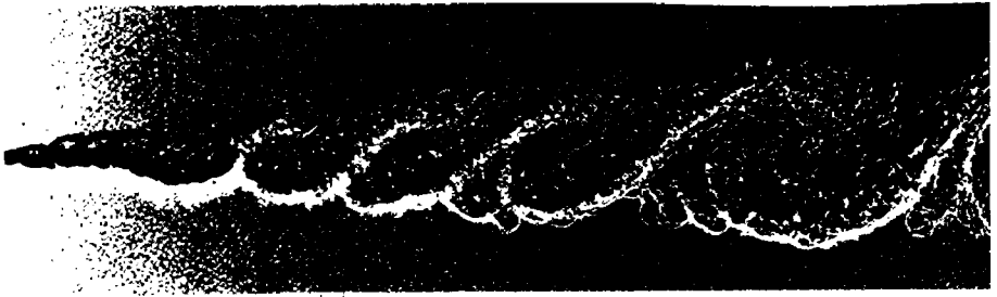
Fig. 5.51. A visualization of the flow of a plane mixing layer. A spark shadow graph of a mixing layer between helium (upper) U_h = 10.1 \text{ m s}^{-1} and nitrogen (lower) U_l = 3.8 \text{ m s}^{-1} at a pressure of 8 atm. (From Brown and Roshko (1974).)
