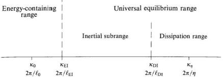
Fig. 6.12. Wavenumbers (on a logarithmic scale) at very high Reynolds number showing the various ranges.
