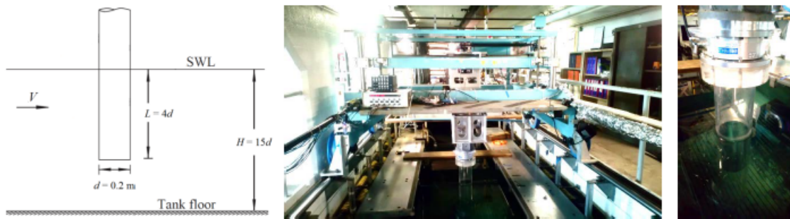
Figure 13 Schematics (left), PMM carriage (middle) and setup for surface piercing truncated cylinder (right)
