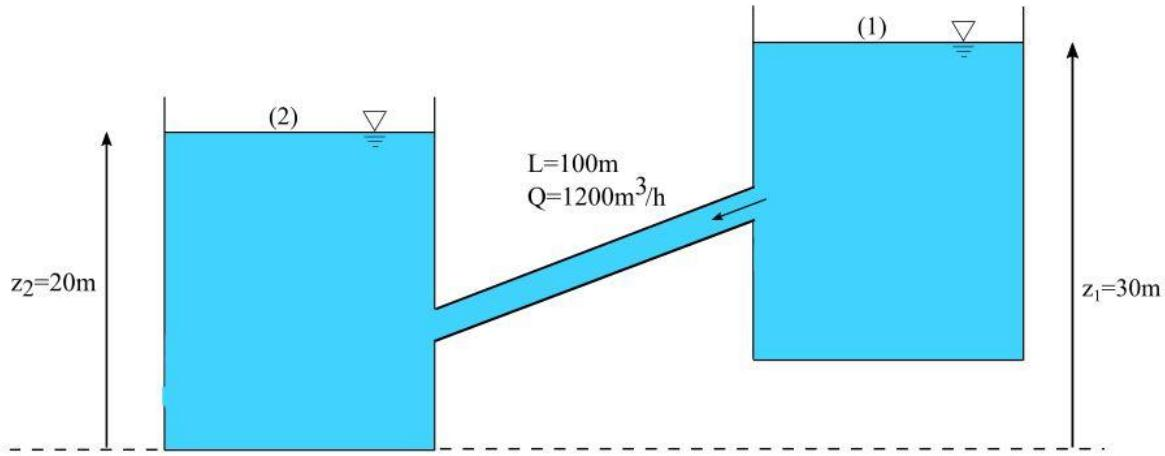
$$\text{Energy equation } \left( \frac{P}{\rho g} + \frac{V^2}{2g} + z \right)_1 = \left( \frac{P}{\rho g} + \frac{V^2}{2g} + z \right)_2 + h_f + h_t$$
