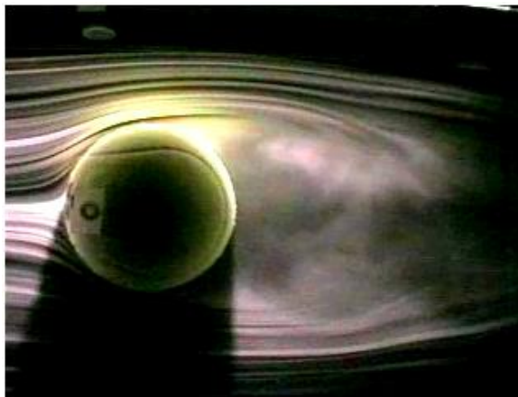
Conditions Producing Separation
