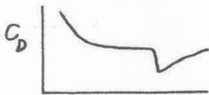
Trial and error solution for  $U$ : Assume  $C_D$ ; obtain  $U$  from Eq.(1),  $Re$  from Eq.(2); check  $C_D$  from Eq.(3), the graph. (3)
