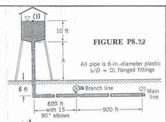
$P_{1} + \frac{V_{1}^{2}}{2g} + Z_{1} = \frac{P_{2}}{8r} + \frac{V_{2}^{2}}{2g} + Z_{2} + (f\frac{l}{D} + \Sigma K_{L})\frac{V^{2}}{2g}, \text{ where } P_{1} = 0, V_{1} = 0, Z_{1} = 16fl+h,$ and  $Z_{2} = 0$  Thus, with  $V = V_{2}$   $16 + h = \frac{P_{2}}{8r} + \frac{V^{2}}{2g} + (f\frac{l}{D} + \Sigma K_{L})\frac{V^{2}}{2g}. \text{ Note: h must be no less than that with}$   $P_{2} = 60psi \text{ and } Q_{2} = 1cfs. \text{ or}$
