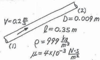
$$\frac{p_1}{\rho} + \frac{V_1^2}{2g} + z_1 = \frac{p_2}{\rho} + \frac{V_2^2}{2g} + z_2 + f \frac{l}{D} \frac{V^2}{2g}, \text{ where } V_1 = V_2 = V \quad (1)$$
