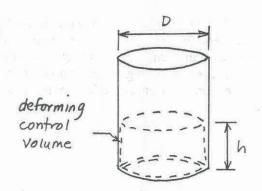
From application of the conservation of mass principle to the control volume containing water only as shown in the figure we have
