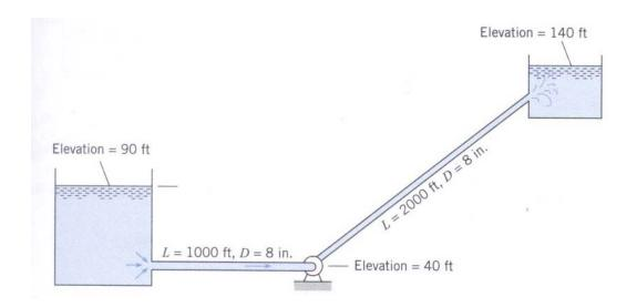
What horsepower must be supplied to the water to pump 3.0cfs at  $68^{\circ}$ F from the lower to the upper reservoir? Assume that the head loss in the pipes is given by  $h_L = 0.015(L/D)(V^2/2g)$ , where L is the length of the pipe in feet and D is the pipe diameter in feet. Sketch the HGL and EGL.
