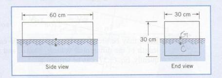
**Solution** First determine the depth of submergence of the block. This is calculated by applying the equation of equilibrium in the vertical direction.
