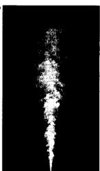
Fig. 1.2. Planar images of concentration in a turbulent jet: (a) Re = 5,000 and (b) Re = 20,000. From Dahm and Dimotakis (1990) .
