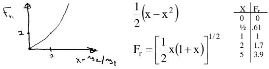
For this particular application we can determine the functional relationship through the use of a control volume analysis: (neglecting  $\mu$  and bottom friction)
