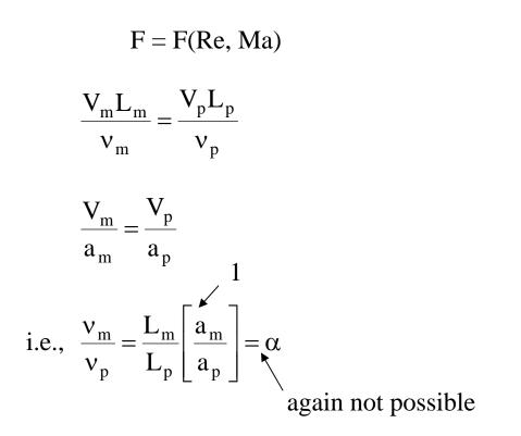
Therefore, in wind tunnel testing Re scaling is also violated
