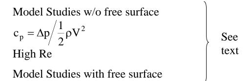
In hydraulics model studies, Fr scaling used, but lack of We similarity can cause problems. Therefore, often models are distorted, i.e. vertical scale is increased by 10 or more compared to horizontal scale
