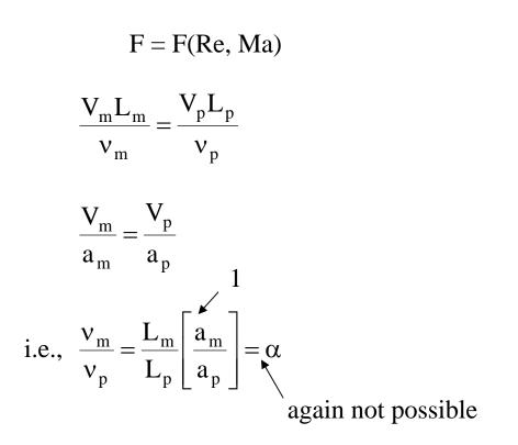
Therefore, in wind tunnel testing Re scaling is also violated
