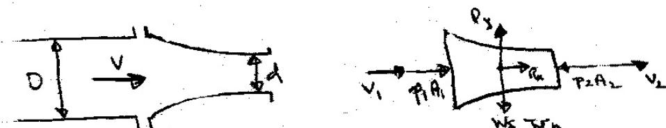
Assume either the pipe velocity or pressure is known. unknown (velocity or pressure) and the exit velocity obtained from combined use of the continuity and Bernoulli equations.
