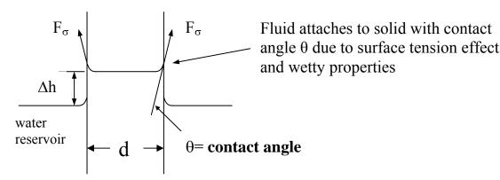
capillary tube d = 1.6mm = 0.0016m  $F_{\sigma} = \sigma \times L$ , L=length of contact line between fluid & solid
