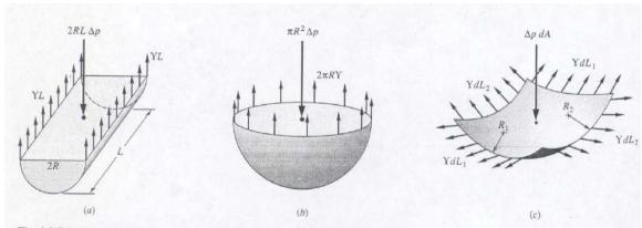
Fig. 1.9 Pressure change across a curved interface due to surface tension: (a) interior of a liquid cylinder; (b) interior of a spherical droplet; (c) general curved interface.
