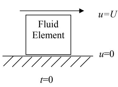
No slip condition: no relative motion between fluid and boundary, i.e., fluid in contact with lower plate is stationary, whereas fluid in contact with upper plate moves at speed  $U$ .
