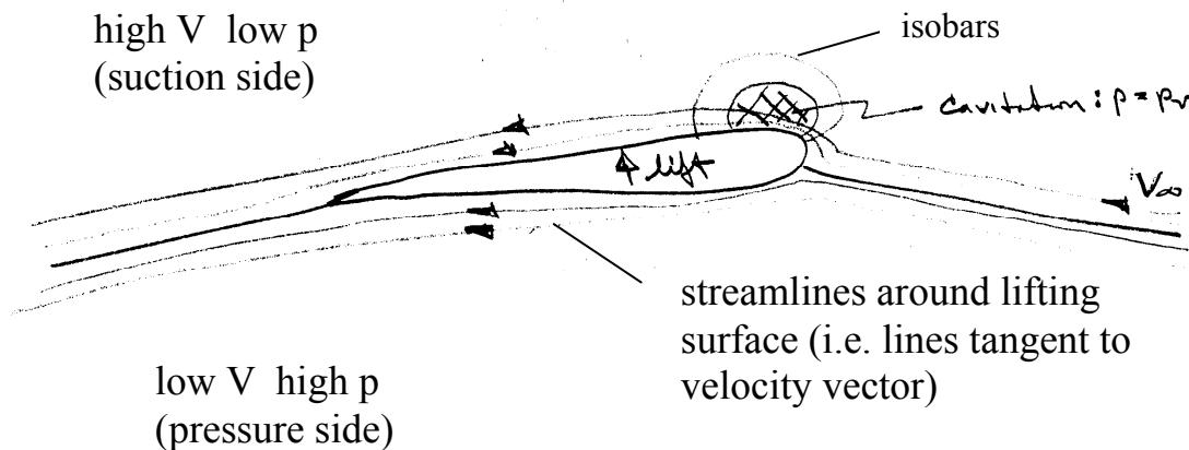
$$\text{Cavitation number} = \frac{p - p_v}{\frac{1}{2} \rho V_\infty^2}$$
