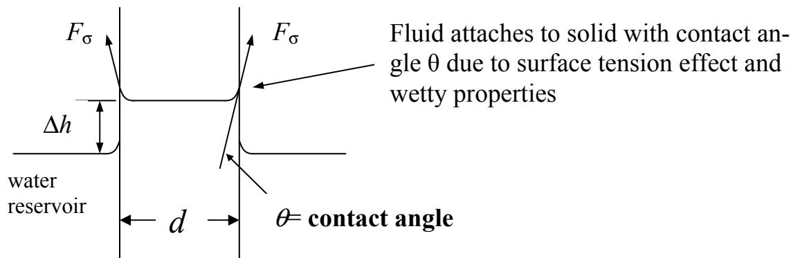
capillary tube  $d = 1.6\text{mm} = 0.0016\text{m}$
