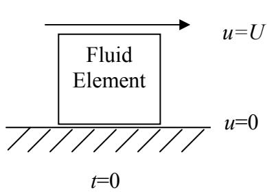
No slip condition: no relative motion between fluid and boundary, i.e., fluid in contact with lower plate is stationary, whereas fluid in contact with upper plate moves at speed  $U$ .
