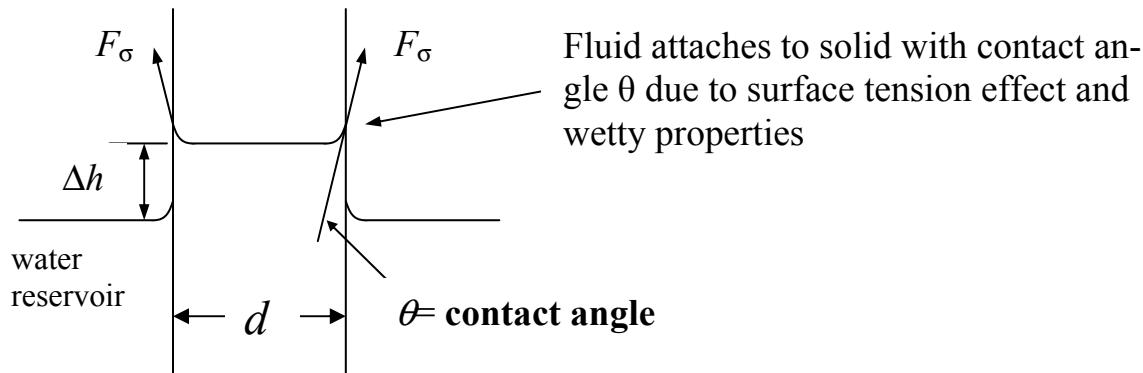
capillary tube  $d = 1.6\text{mm} = 0.0016\text{m}$
