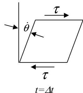
Fluid deforms, i.e., undergoes rate of strain  $\dot{\theta}$  due to shear stress  $\tau$
