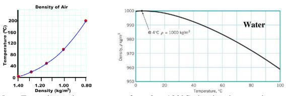
Note: For a change in temperature from 0 to 100°C, density changes about 29% for air while only about 4% for water.
