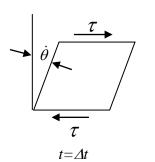
No slip condition: no relative motion between fluid and boundary, i.e., fluid in contact with lower plate is stationary, whereas fluid in contact with upper plate moves at speed *U*.
