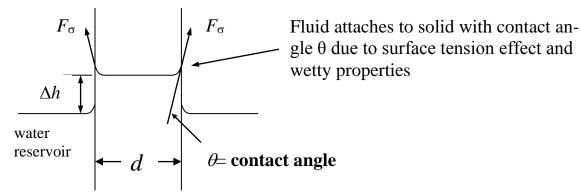
**Example:** Capillary tube d = 1.6mm = 0.0016m  $F_{\sigma} = \sigma \times L$ , L=length of contact line between fluid & solid (i.e.,  $L = \pi D$  = circumference)
