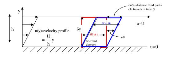
Newtonian fluid:  $\tau = \mu \dot{\theta} = \mu \frac{\delta \theta}{\delta t}$  $\tan \delta \theta = \frac{\delta u \delta t}{\delta y}$  or  $\delta \theta = \frac{\delta u \delta t}{\delta y}$  for small  $\delta \theta$
