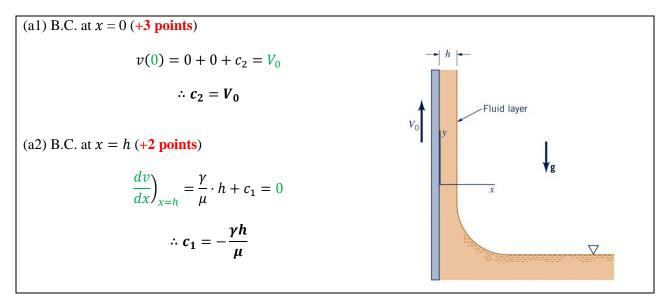
(b1) Shear stress (+3 points)  $\tau_{w} = \mu \frac{dv}{dx} \Big|_{x=0} = \mu \left( \frac{\gamma}{\mu} x - \frac{\gamma h}{\mu} \right)_{x=0} = -\gamma h = (12.4 \times 10^{3})(0.002) = -24.8 \text{ N/m}^{2}$ (b2) Flow rate (+2 points)  $q = \int_{0}^{h} v dx = V_{0}h - \frac{\gamma h^{3}}{3\mu} = (0.015)(0.002) - \frac{(12.4 \times 10^{3})(0.002)^{3}}{3(1.5)} = 7.96 \times 10^{-6} \text{ m}^{3}/\text{s}$   $\approx 8 \text{ cm}^{3}/\text{s}$  4. [Pipe flow - *Q*]
