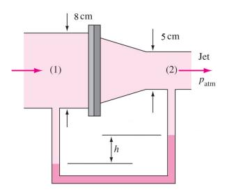
$$\therefore V_1 = \sqrt{\frac{(2)(71,300 \text{ Pa})}{(999 \text{ kg/m}^3) \left[ \left( \frac{0.08 \text{ m}}{0.05 \text{ m}} \right)^4 - 1 \right]}} = 5.1 \text{ m/s}$$
