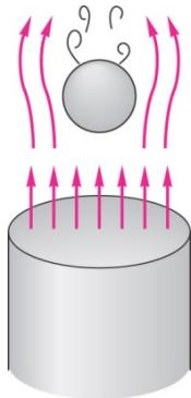
The ball weight must balance its drag:
