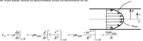
Note that the quantity du/dr is negative in pipe flow, and the negative sign is added to the  $\tau_w$  relation for pipes to make shear stress in the positive (flow) direction a positive quantity. (Or, du/dr = -du/dy since y = R - r). Then the friction drag force exerted by the fluid on the inner surface of the pipe becomes
