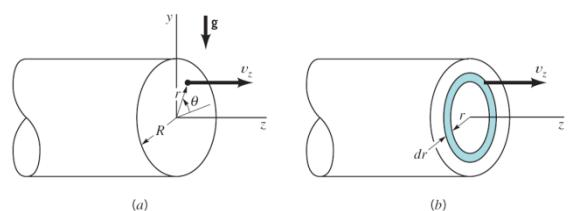
$$1) \text{ Flow rate: } Q = \int_0^R v_z dA = -\frac{\pi R^4}{8\mu} \left( \frac{\partial p}{\partial z} \right) = \frac{\pi R^4 \Delta p}{8\mu \ell} \quad \therefore -\frac{\partial p}{\partial z} = \frac{\Delta p}{\ell}$$
