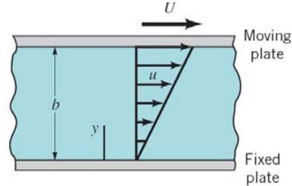
$$\text{Shear stress at the bottom wall: } \tau_w = \mu \frac{du}{dy} \Big|_{y=0} = \frac{\mu U}{b}$$
