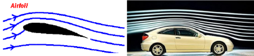
Examples of streamlines around an airfoil (left) and a car (right)
