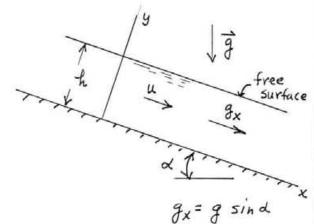
With the coordinate system shown in the figure v=0, w=0, and from the continuity equation  $\frac{\partial u}{\partial x}=0$ . Thus, from the x-component of the Navier-Stokes equations (Eq. 6.127a)
