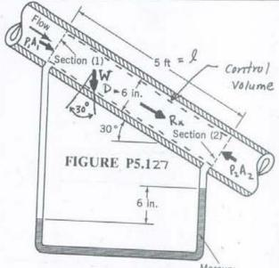
(a) The difference in pressure, P. - Pz, may be obtained from the manometer (see Section 2.6) with the fluid statics equation
