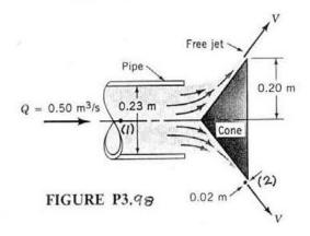
$$\frac{p_1}{\gamma} + \frac{V_1^2}{2g} + z_1 = \frac{p_2}{\gamma} + \frac{V_2^2}{2g} + z_2$$
