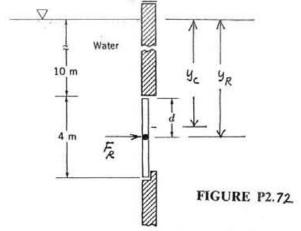
(a) As depth increases the center of pressure moves toward the centroid of the gate. If we locate hinge at ye when depth = 10m +d, the gate will open automatically for any further increase in depth.
