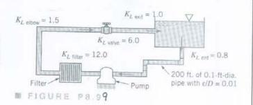
$$\frac{\rho_{l}}{8} + Z_{l} + \frac{V_{l}^{2}}{2g} + h_{p} = \frac{\rho_{2}}{8} + Z_{2} + \frac{V_{2}^{2}}{2g} + (f \frac{1}{D} + \sum_{i} K_{L_{i}}) \frac{V^{2}}{2g}$$
