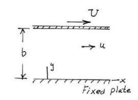
(a) For steady flow with v=w=0 it follows that the Navier-Stokes equations reduce to (in direction of flow)  $0=-\frac{\partial P}{\partial x}+\mu\left(\frac{\partial^2 u}{\partial y^2}\right) \qquad (Eg. 6.129)$
