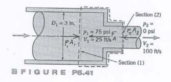
For this problem we include in the control volume the nozzle as well as the water at an instant between sections (1) and (2) as indicated in the sketch above. The horizontal forces acting on the contents of the control volume are shown in the sketch. Note that the atmospheric forces cancel out and are not shown. Application of the horizontal or x-direction component of the linear momentum equation (Eq. 5.22) to the flow through this control volume yields
