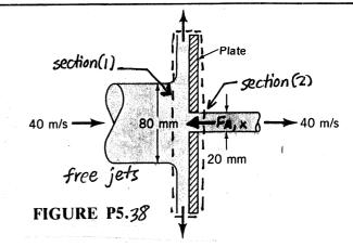
The control volume contains the plate and flowing air as indicated in the sketch above. Application of the hovizontal or X direction component of the linear momentum equation yields
